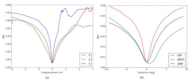
Fig. 8. NID values at varying offsets from the ground truth pose. These plots are averaged across 20 different locations. (a) Translational axes with x, y and z shown as red, green and blue respectively. (b) Rotational axes with roll, pitch and yaw shown as red, green and blue respectively. The second local minimum in the z axis is due to the road looking very similar when rendered from below as it does from above.
