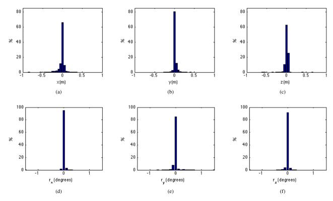
Fig. 7. Histograms showing displacement between the localised solution and ground truth in each degree of freedom. The coordinate system places x in the direction of the vehicle's travel, y to the vehicle's right, and z downwards into the road.
