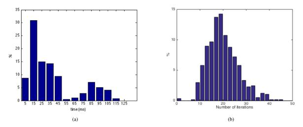
Fig. 9. Runtime behaviour of optimiser. (a) Time taken to evaluate the NID function, including rendering the synthetic image. The majority of cost function evaluations take less than 25 ms. (b) Number of cost function evaluations carried out in each optimisation. Most optimisations require approximately 20 evaluations.
