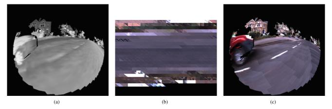
Fig. 2. Generation of the prior: (a) First we build a mesh by stitching together subsequent scans from the push-broom LIDAR; (b) we then project the mesh in turn into each camera image, and generate a texture for each triangle — here we show all the textures for a single 'slice,' from many different input images; and (c) we combine all the slices with their textures for the final prior.
