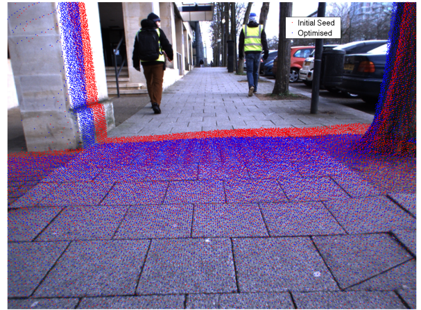
Fig. 9: Solution Quality: Fig. shows the projection of a 3D point cloud on a reference image. The red dots show the non-optimal initial-seed, and the blue dots show the optimised solution for \mathbf{g}_{C_{aL}} . The displayed solution is obtained after 10 iterations of the alternating method, and shows considerable improvement on visual inspection.
