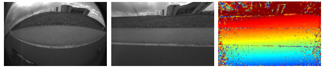
Fig. 6. Depth map computation—perspective images (middle) are rendered from the fisheye images (left) and plane sweep stereo matching is used between three temporally consecutive images to produce a depth map (right) for each camera at each time.
