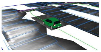
Fig. 1: The semantic information placed relative to the metric map. Shown are the driving lanes in green, and the parking spaces in blue.
