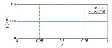
Fig. 2: The likelihood of making an error given some measurement z (or *error function*) for two idealised classifiers, given by Figure 1. The *uniform* classifier is non-introspective because the likelihood of error is not correlated with classification confidence  $H_N(z)$  (see (4) from the original paper), and thus is not introspective. The *optimal* classifier has the same overall error rate, but makes all of its mistakes with high uncertainty, and is therefore more introspective.
