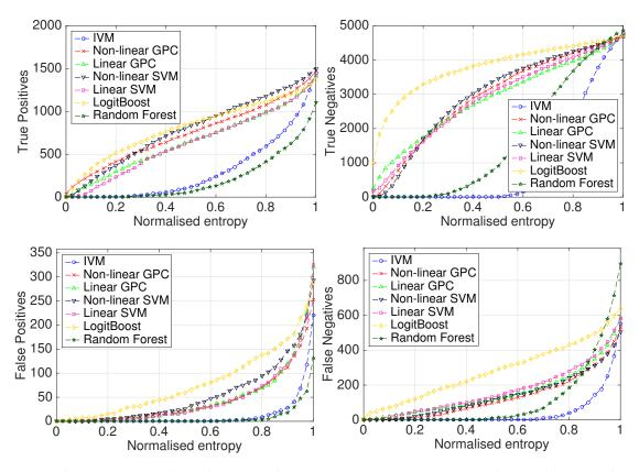
Fig. 9: Cumulative frequency plots of classification confusion (true positives, true negatives, false positives, and false negatives) against normalised entropy (uncertainty), using the KITTI data set. The classifiers are trained on 200 and 500 instances of pedestrians and background respectively, and are tested on 2,000 and 5,000 of those classes. See the caption for Figure 7 for more detail. (Best viewed in colour.)
