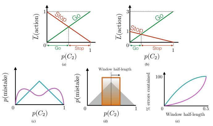
Fig. 4: (a) We have set equal cost to a false positive (take the *stop* action when there is, in fact, no person:  $C_1$ ) and the false negative (take the *go* action when there is a person:  $C_2$ ). The expected losses from the two actions meet at  $p(C_1) = p(C_2) = 0.5$ , and choose the action which minimises the expected loss.
