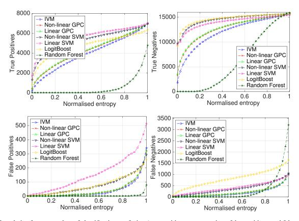
Fig. 8: Cumulative frequency plots of classification confusion (true positives, true negatives, false positives, and false negatives) against normalised entropy (uncertainty), using the Daimler Pedestrian data set. The classifiers are trained on 250 and 500 instances of pedestrians and background respectively, and are tested on 8,000 and 16,000 of those classes. See the caption for Figure 7 for more detail. (Best viewed in colour.)
