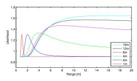
Fig. 4. Inverse Depth-parameterized likelihood function evaluated for a variety of nominal model depths. This parameterization evaluates highrange depth points with higher variance than shorter ranges - accurately representing the underlying disparity measurement uncertainty.
