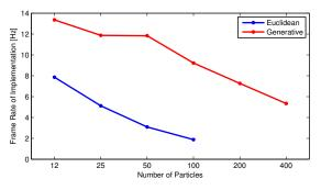
Fig. 10. Timing statistics for both likelihood functions. In the case of the later, real time operation (at 10Hz) has be achieved with 100 particles and the frequency reduces linearly with the number of particles.
