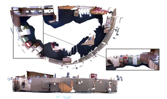
Figure 19: Dataset of a small coffee room. Inset shows everyday objects such as bins and fridges are captured in high detail and how the deformation approach works well in smaller environments.
