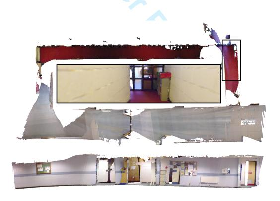
Figure 20: Corridor loop closure dataset. The inset shows map consistency at the point of loop closure. Extension 1 shows the actual map correcting deformation occurring.
