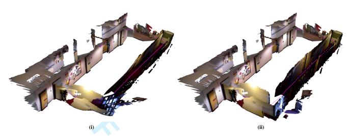
Figure 12: From left to right; (i) Highly distorted map produced when a naïve nearest neighbour sampling and connectivity strategy is used; (ii) Non-distorted map loop closure using our proposed sampling and connectivity strategy.
