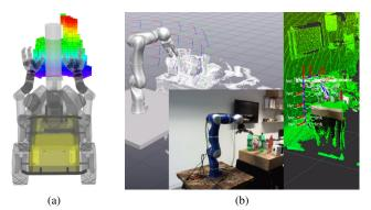
Fig. 4. Scene representations during the experiments: (a) Bimanual mobile manipulator with octomap used for planning, (b) Dual representation for fixed-base manipulator: Dense, visual map for segmentation shown on the left, and octomap for planning to the right.
