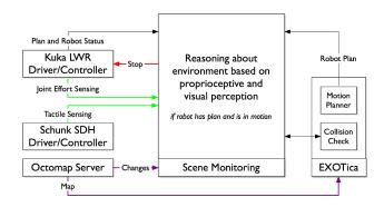
Fig. 5. The implemented scene monitoring utilizing different perception modalities: visual RGB-D data, tactile, and joint effort sensing. Diagram showing modules active during Experiment 1 (Kuka LWR).
