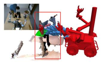
Fig. 11. The scene monitoring continuously integrates fused and filtered sensor data in an OctoMap and reasons about changes: Here, a human reaches into the robot workspace crossing the planned trajectory (shown in blue), and the robot halts execution (robot state shown in red).
