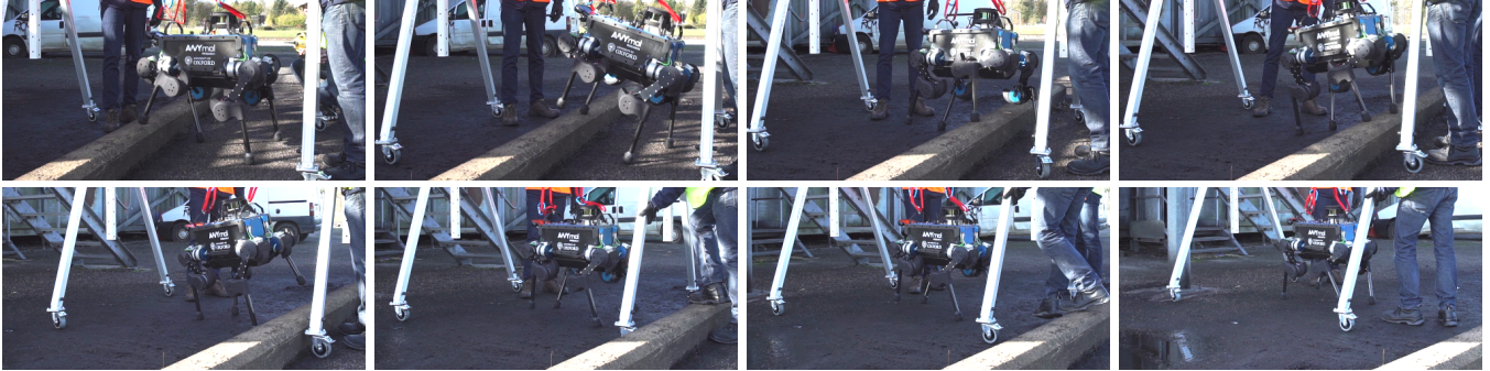
Fig. 6: Utopian trajectory executed on the real robot and oil rig scenario. Left to right and top to bottom: footsteps over slab, then fast trotting towards goal.
