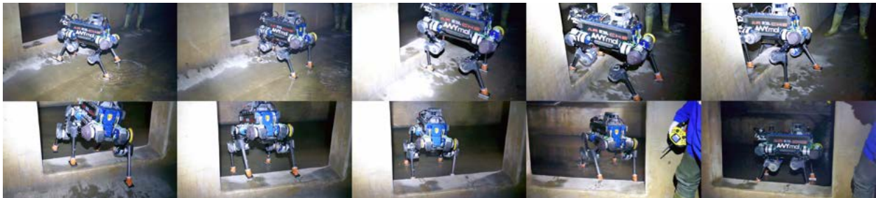
(e) The robot performing the crossing maneuver during mission 4. The robot has climbed onto the threshold and is transiting from tunnel two to tunnel one to continue the inspection.
