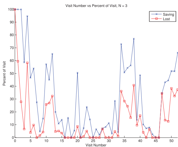
Fig. 17. Performance results for N = 3 , with the percentage of each visit that was spent saving and lost shown. The system saved 31.95% of all of the possible experiences and was lost 14.12% of the time.
