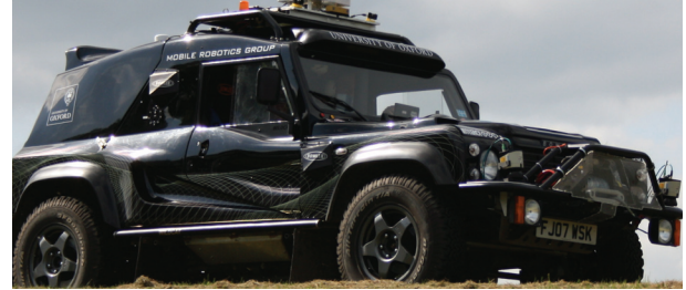
Fig. 6. The group's vehicle, the Wildcat, was used to collect 37km of visual data. The vehicle is equipped with a range of sensors including cameras, lasers and an INS. It also houses a high-end computer.
