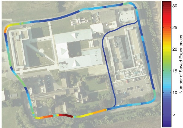
Fig. 7. Overhead of the two routes visited during data collection. The outer loop, indicated by the thicker line, was driven 47 times, while the inner loop, shown by the thinner line, was driven 6 times. The intensity of the trace shows how many experiences have been laid down at each point. See Figure 8, 9, 10 and 11 for examples of places with low and high experience density.
