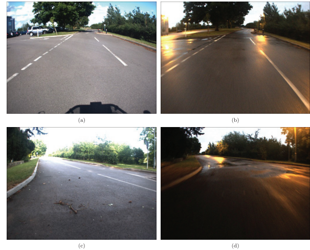
Fig. 15. Examples of localisation failure leading to the creation of new saved experiences on visit 38: (a), (c) from previously saved experiences; (b), (d) from the live stream.
