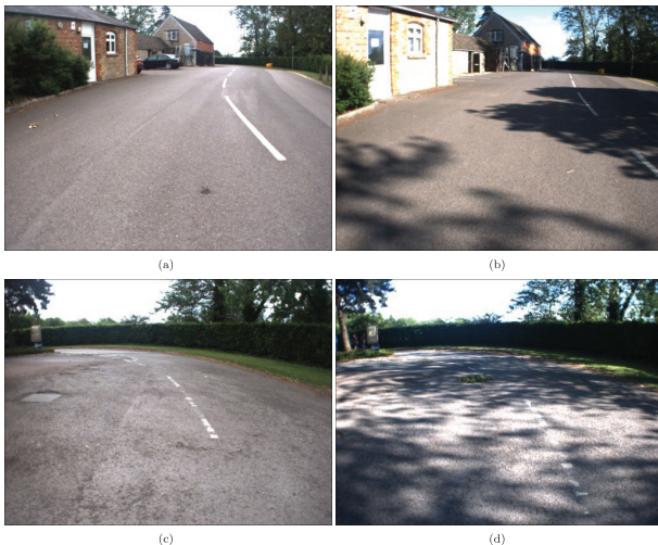
Fig. 14. Examples of localisation failure leading to the creation of new saved experiences on visit 4: (a), (c) from previously saved experiences; (b), (d) from the live stream.
