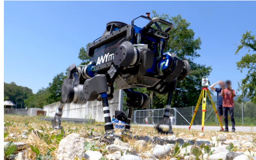
Fig. 1. ANYmal trotting over a field of small rocks at the Swiss Military Rescue Centre in Wangen an der Aare (Switzerland). The ground truth was collected using a Leica TS16 laser tracker (visible in the background). Video: http://youtu.be/w1Sx6dIqqQo
