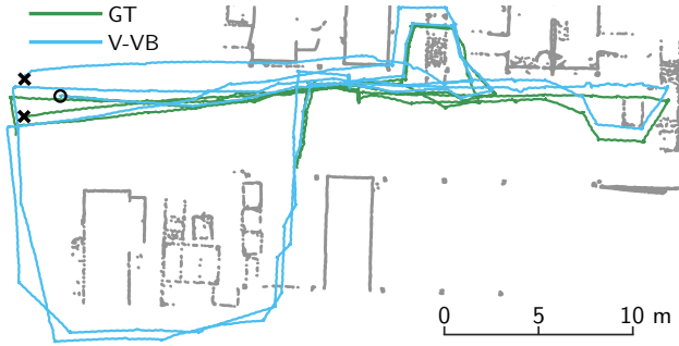
Fig. 7. Aerial view of the trajectories for method V-VB and the ground truth on the FSC dataset (240 m traveled). The common start point is indicated with a circle and the two endpoints with a cross. The lower part of the trajectory has no ground truth. Note that V-VB has no loop-closure system.
