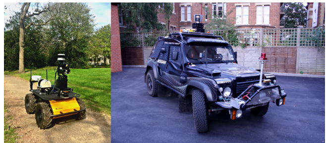
Fig. 5: The robots utilised to collect data for our experiments. A Clearpath Husky robot (left) was used to collect the GS dataset with a push-broom LIDAR and a Multisense SL. A Bowler Wildcat platform (right) was utilised to collect the CP dataset, equipped with a Velodyne HDL-32E LIDAR, OxtS GPS, Novatel INS and Bumblebee2 camera.
