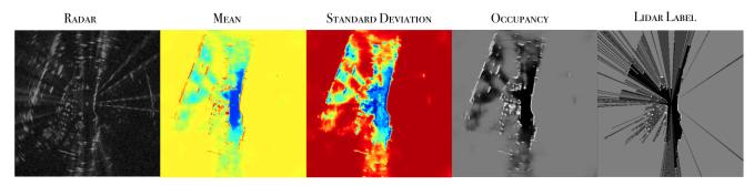
(c) Our model successfully identifies occupied free and occluded space in challenging real world environments.
