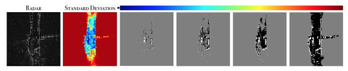
(d) A scene segmented as predicted occupied (white), unoccupied (black) and unknown (grey) for decreasing confidence thresholds (left to right) on the predicted standard deviation  $\gamma_{\phi}$ . From most certain to most least certain, we move from high power returns labelled as occupied, to a region nearby and up to the first return, to space that lies in partial and full occlusion.
