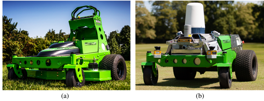
Fig. 1 Photos of the platform before (a) and after (b) modifications. The modifications are clearly visible with the sensors at the front and the power and control circuitry compartment at the rear
