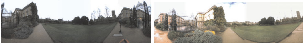
Fig. 7. Example place recognition result generated by FAB-MAP under markedly different lighting conditions. Probability of loop closure is calculated to be 0.9519.
