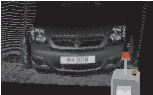
Fig. 21. Close detail of a point cloud built by rendering range and reflectance data from the estimated trajectory of a moving Segway platform (New College dataset).
