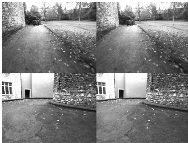
Fig. 14. FAB-MAP false positive rejected by stereo registration due to lack of correspondences. The two scenes are clearly not identical although they do share a common appearance.
